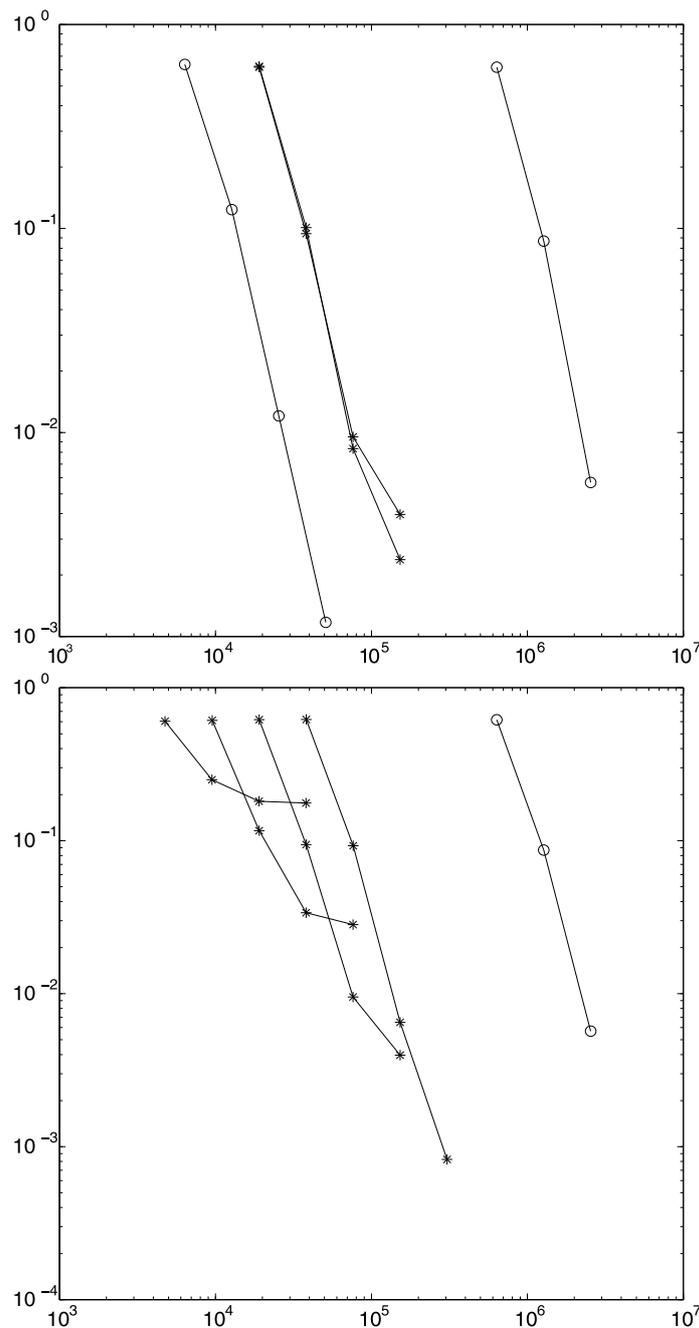
**Fig. 6.** Efficiency diagrams for SAM applied to the GGL formulation of double pendulum equations. The circles correspond to standard integration with HERK3. The stars to SAM with HERK3 as macro- and micro-integrator. On the top panel, different lines correspond to different values of  $\epsilon$  and a fixed macro-step-size  $H = \pi/2500$ . On the bottom panel  $\epsilon = 10^{-6}$  and different lines correspond to different macro-step-sizes  $H = \pi/625, \pi/1250, \pi/2500, \pi/5000$ .
