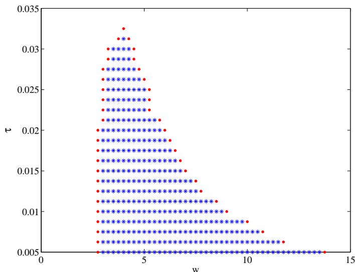
FIGURE 2. Combinations of  $\tau$  and  $w$  that ensure stabilization. Experimental results.
