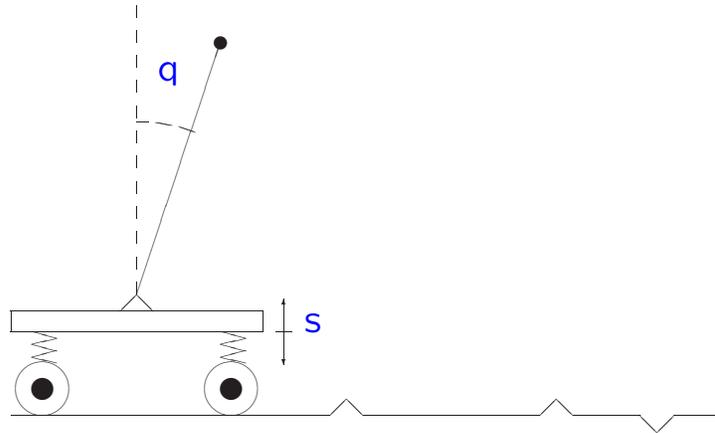
FIGURE 1. The inverted pendulum on a carriage that travels on a bumpy road.
